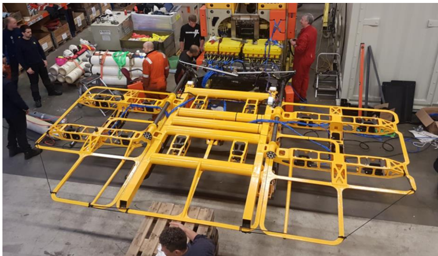
UltraTEM Marine system as configured for Boskalis and marketed as the SubTEM-ROV
