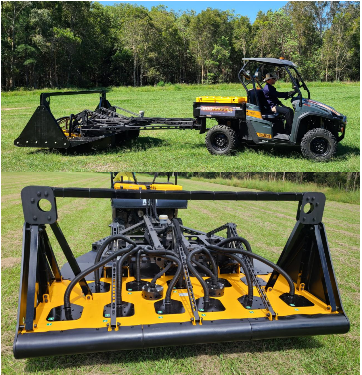
FIGURE 4. TOWED-ARRAY CLASSIFIER (TNB).
