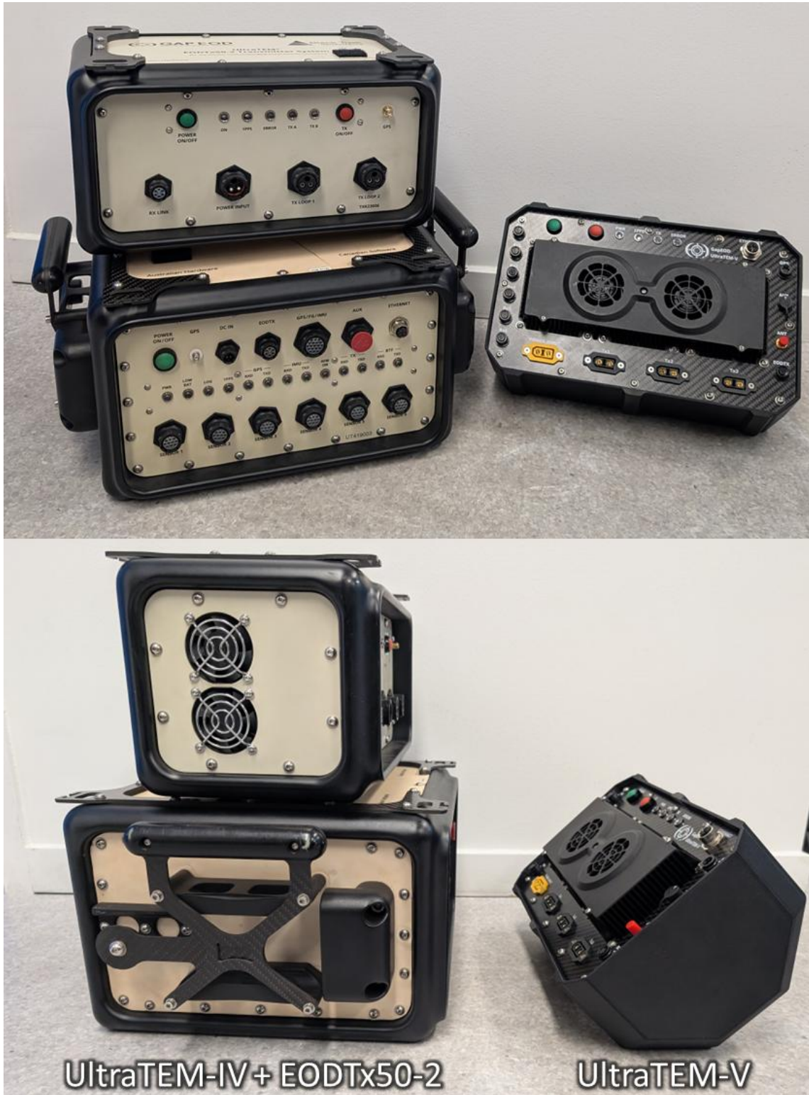
FIGURE 3 ULTRATEM-IV RECEIVER BANK AND EODTx50-2 TRANSMITTER (LEFT) COMPARED TO AN ULTRATEM-V RECEIVER BANK (RIGHT).
