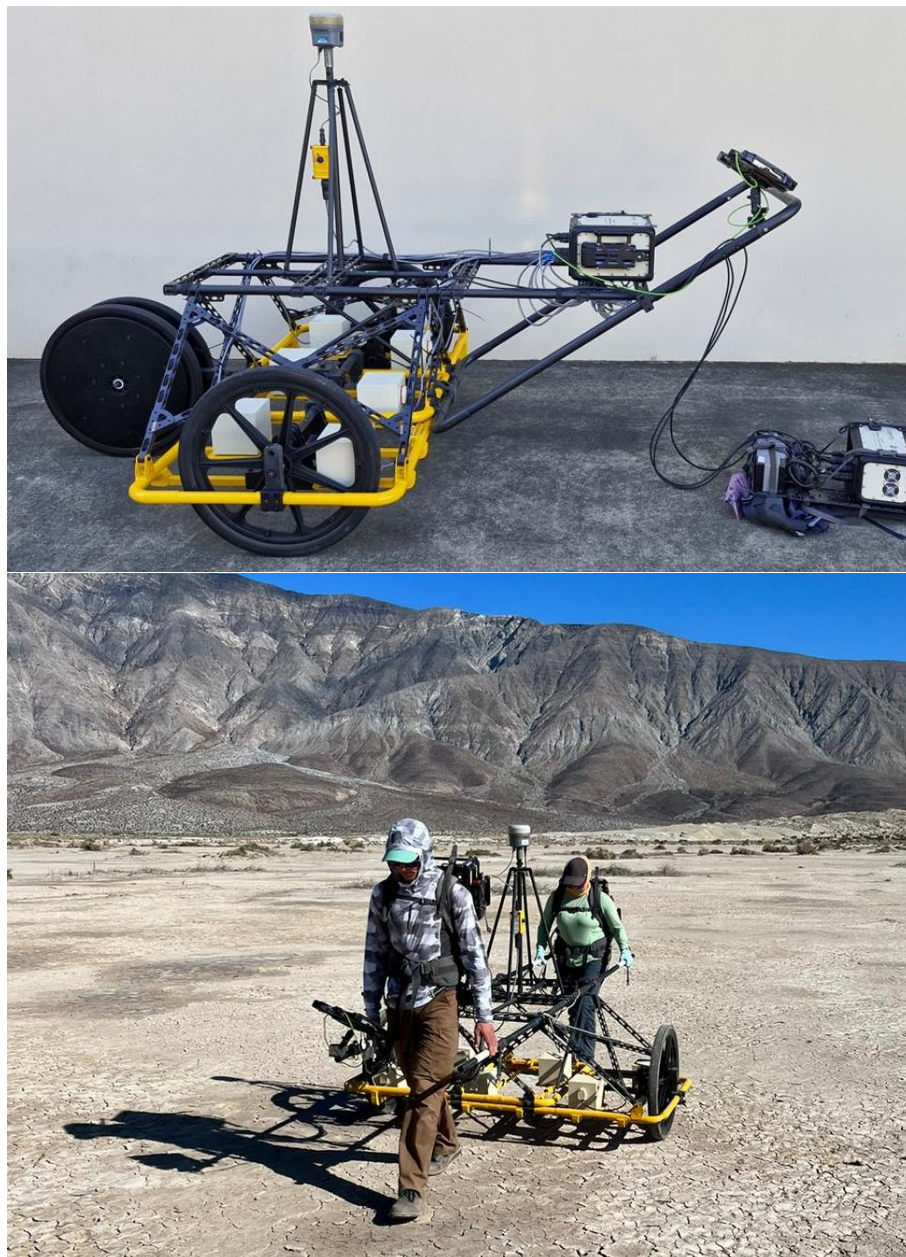
FIGURE 6 PEDESTRIAN CLASSIFIER (TNC) SYSTEM CONFIGURATIONS. PUSH-CART (TOP), HYBRID (BOTTOM).
