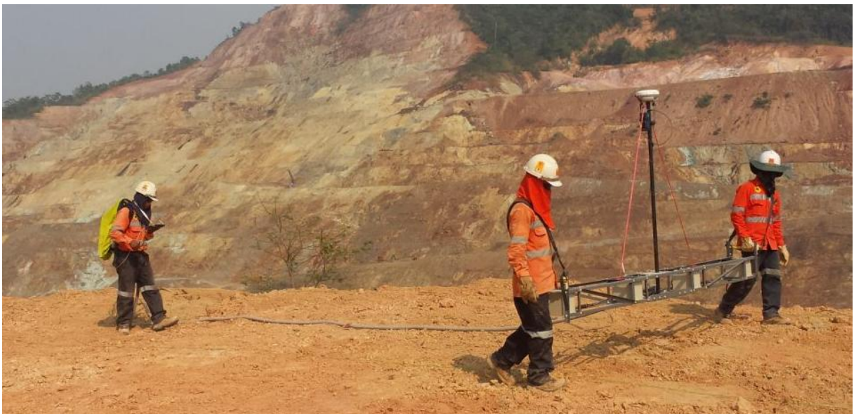
FIGURE 9. ULTRATEM DEEP SEARCH SYSTEM IN OPERATION IN LAOS.
