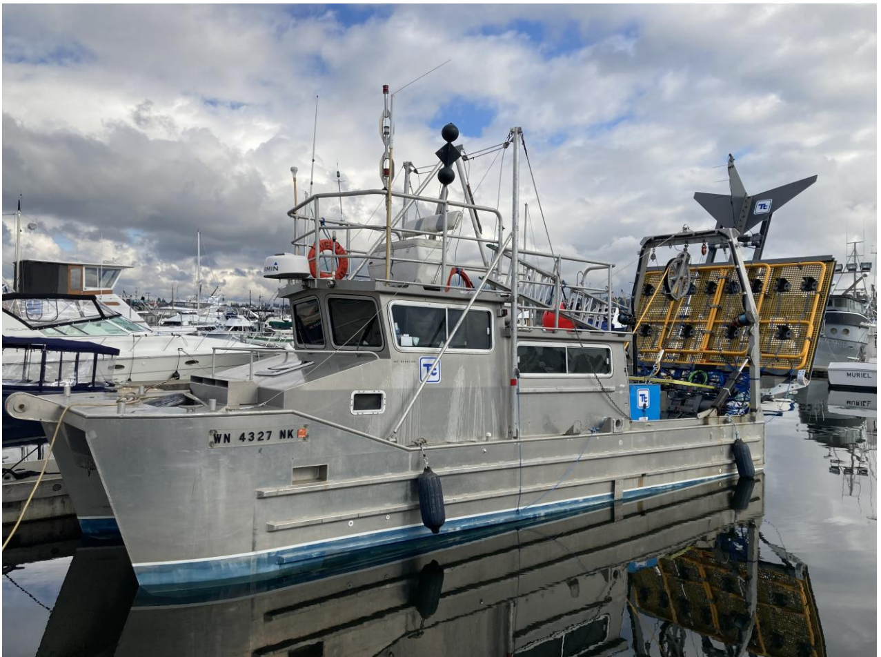
FIGURE 17. THE ULTRATEM MARINE SYSTEM INSTALLED ON A NON-METALLIC SLEDGE TOWED BEHIND A SMALL BOAT.
