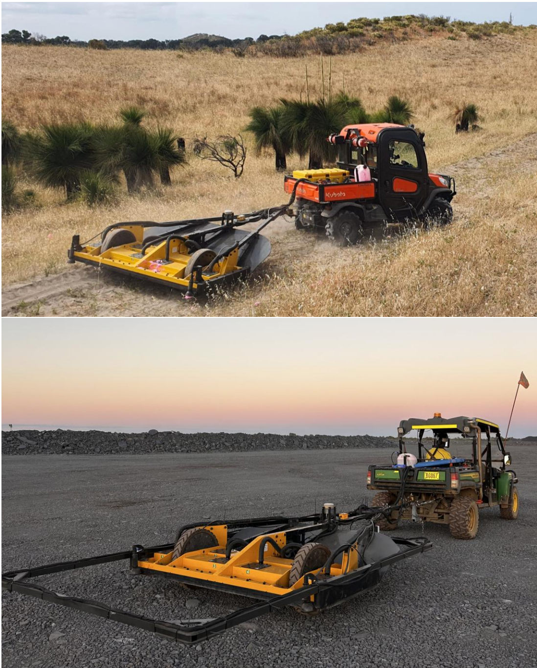
FIGURE 5 TOWED-ARRAY SCREENER (TPC) CONFIGURATIONS. STANDARD (TOP) & 3 RD TX LOOP (BOTTOM).
